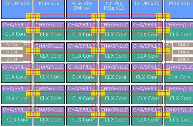
Figure 2: Cascade Lake Processor Architecture [17]
